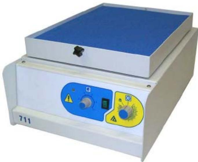
VDRL Stirrer **ES-711 +** with orbital rotating oscillating plate, is suitable for microflocculation tests, latex tests, cellculture, decoloration of electrophoresis strips. Electronic regulation of oscillation in range 50 to 250 per minute. Oscillation amplitude 32 mm.
